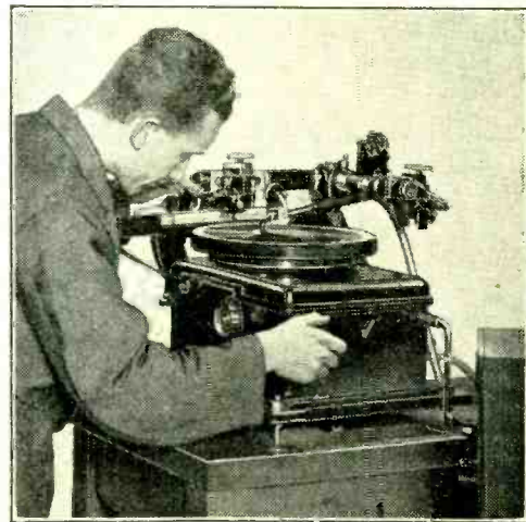
H.M.V. disc recording apparatus used in their studios at St. John's Wood.
